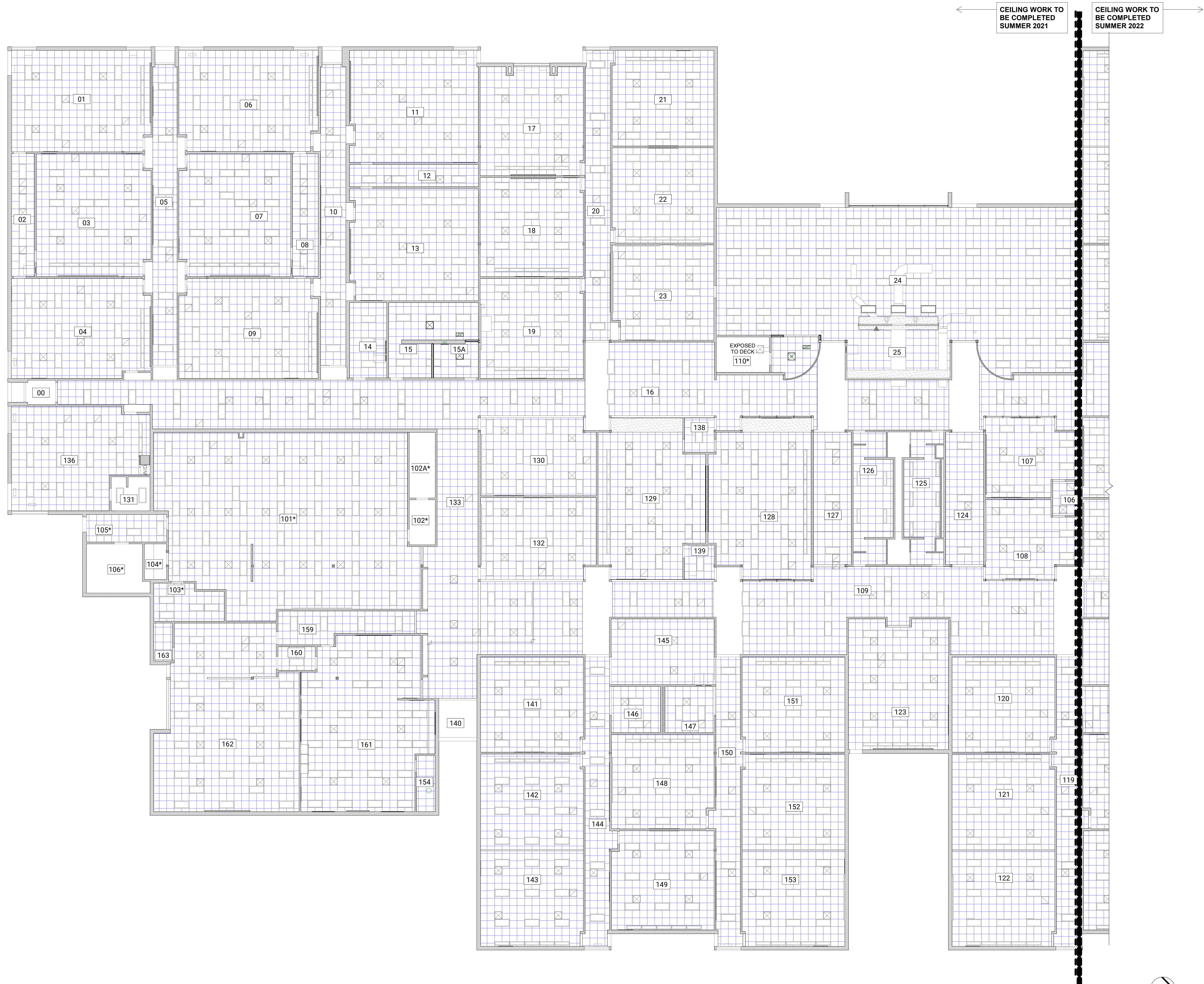
① REFLECTED CEILING PLAN - AREA 'A' CD BOE 3/32" = 1'-0"
